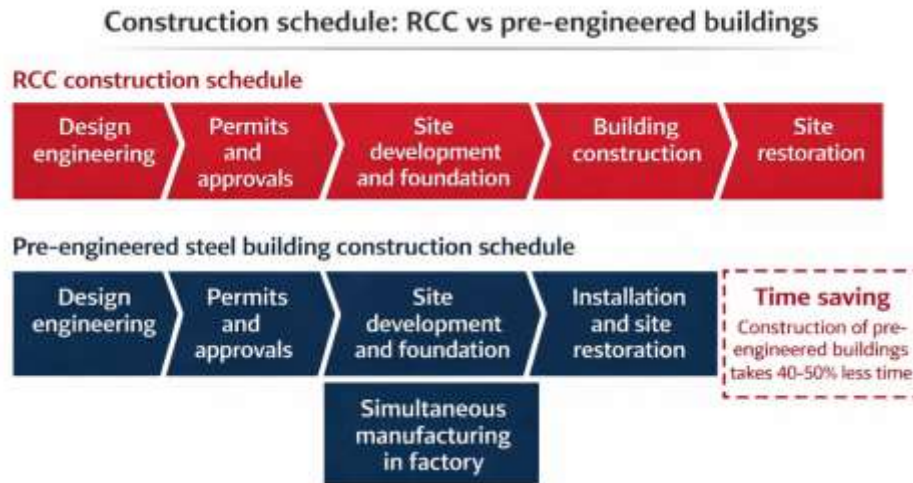
Exhibit 44: PEB vs RCC – Construction time saved more than overcomes the initial higher construction cost
